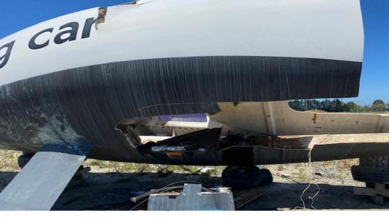
broken. The boat had sustained a fatal blow to the port side – through the side deck and rear bulkhead splitting the cabin top and causing stress cracks in the cockpit floor. Her time on the bottom was evidenced by the thick mud throughout the interior. However, the mast lay shining in the Canterbury sun with the beautiful carbon twill evident below the clear coat. Just what I was wanting.
