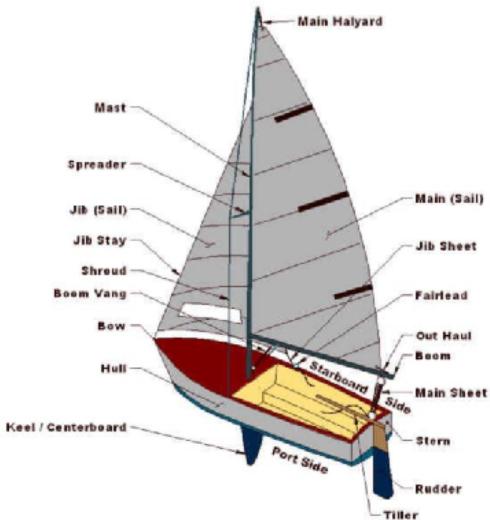
When sailing the boat often leans over, or “**heels**”, due to the force of the wind on the sails. Single-hull boats don’t get pushed completely over though due to the weight of the **keel** underneath the **hull** which counteracts the force of the wind.
